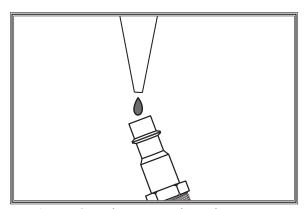
**Figure 3.** Lubricating directly into air fitting.
